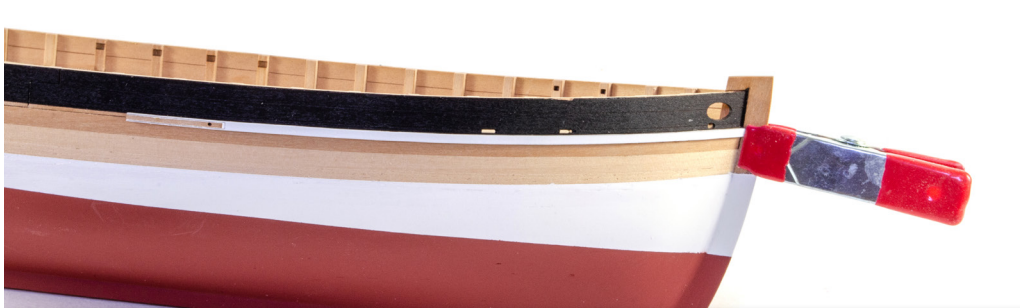
131. The forward section of each rail can now be applied to the hull. This sits directly underneath the black bulwark area. (left-hand side shown).
