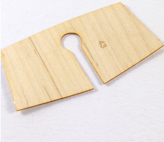
58. Glue this into position as shown here, with the narrow edge meeting the stern timbers at the point where they change angle. Maple veneer is very easy to bend. You may wish to glue the narrow edge first and then leave to dry before forming the wider edge against the underside/bulkhead #13.
