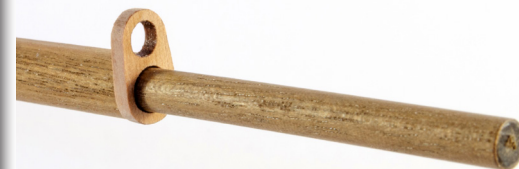
208. From the 1.5mm wood sheet, remove one part #95 and glue into position as seen here so the part sits snug into the shoulder where you reduced the dowel diameter.
