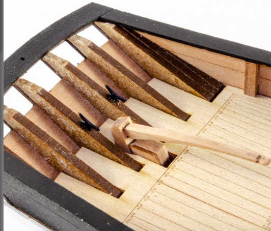
188. From the 0.4mm photo etched sheet, remove the cleats #PE-17 and glue into place on the two innermost stern timbers. Paint the parts black.
