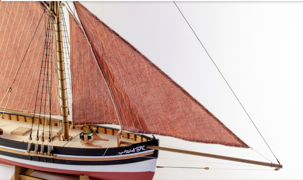
231. The upper jib can now be fitted. This is very easy. Use the plan and photo as an approximation of the sail position.
