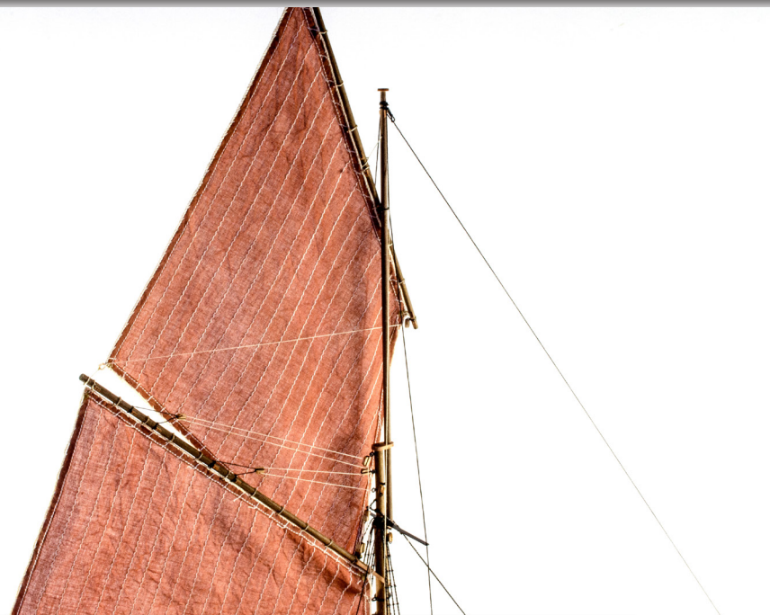
229. And here you see the position of the top sail in relation to the main sail.
