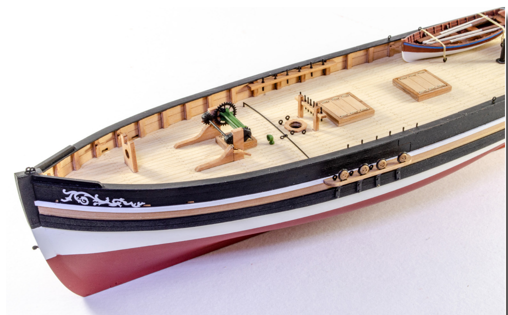
203. The boat is now lashed to the deck via the four eyelets and some 0.25mm natural thread. In these photos you can see the completed deck works.
