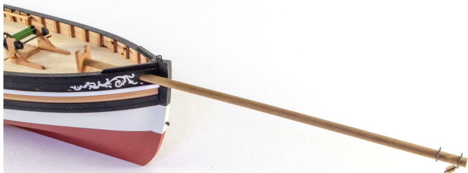
206. Slot the bowsprit into position so the inner end is only just through the support block. Note the correct orientation of PE and block at the outer end.
