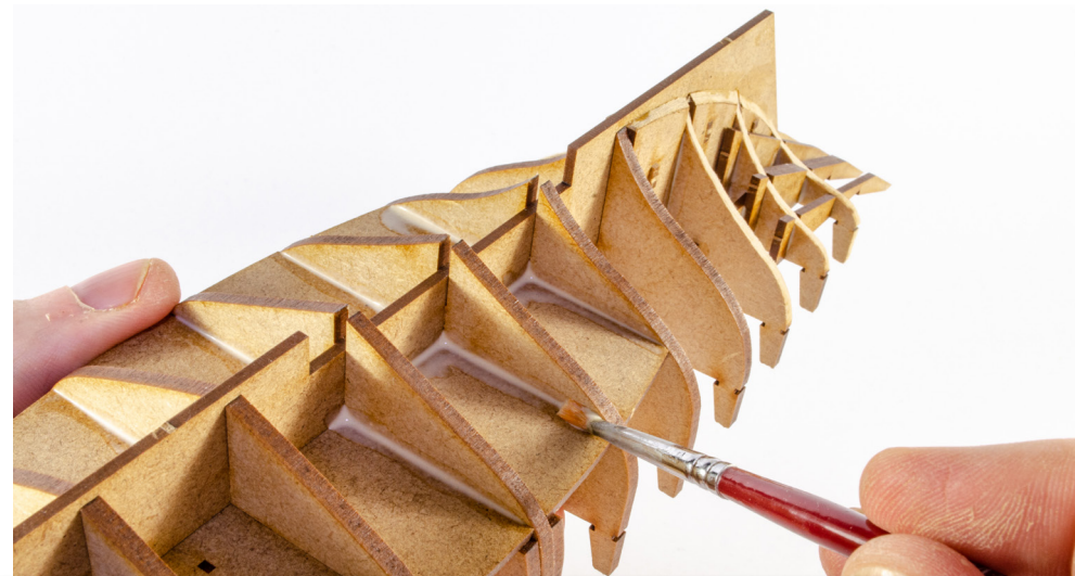
40. Make sure that everything is pushed firmly together, and nothing is misaligned. Now, brush slightly diluted wood glue into the various slots and joints around the hull. Once done, leave to dry for a few hours.
