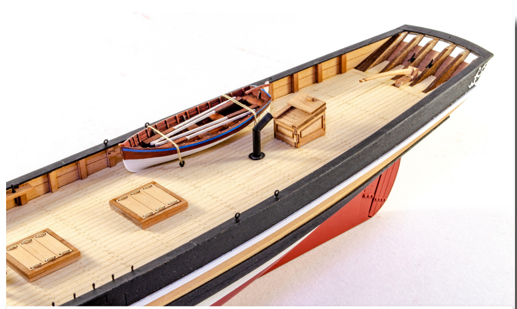
203. The boat is now lashed to the deck via the four eyelets and some 0.25mm natural thread. In these photos you can see the completed deck works.
