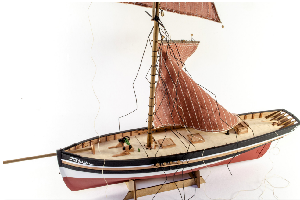
219. We now need to add the shroud lines, as per plan. These are from 0.75mm black thread. These are added in pairs, on alternate sides, each time.
