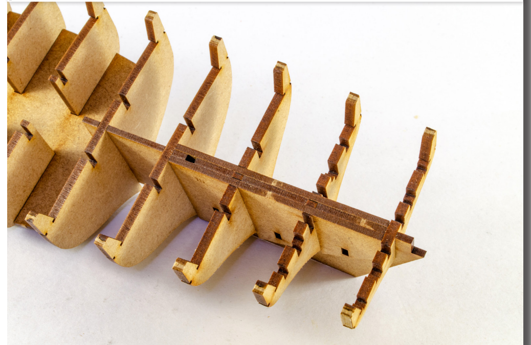
25. Slide part #15 into place as shown, gluing it only to the keel and not the bulkheads. You will see here that the part slots into the top of the bulkheads #11 and #12 and against the keel itself. Repeat with part #16.
