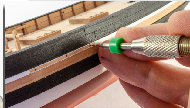
197. Drill the accompanying holes in the outer rails, about 2mm deep, taking into account the thickness of the rail into that calculation.
