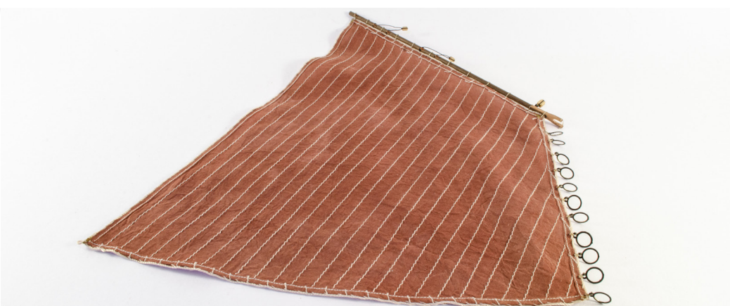
214. If you are using sails, then you need to stitch the main gaff to the largest sail, as shown and also stitch the main sail rings (PE-16) to the sail. Add the other rig lines
