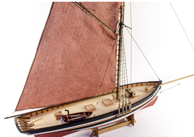
228. This photo gives you a good idea about how the main sail is rigged, with position of the sail on the mast.
