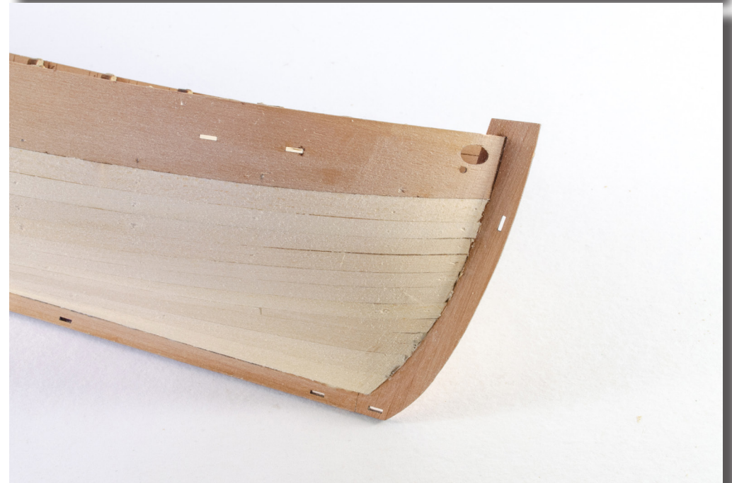
72. Once you've removed all your brass pins, you will now need to sand the hull smooth. Use a grade of paper around 110 grit, or similar. Finish the hull in something a little finer once you have about completed the sanding.
