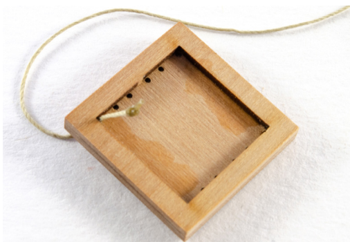
156. This applies to all assemblies you've just made. Use a length of 0.5mm natural thread and tie a knot in one end. Apply some CA to the opposite end and trim to a point. Thread the pointed end through the corner hole, from the underside.
