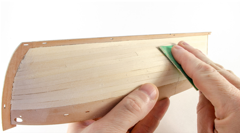
72. Once you've removed all your brass pins, you will now need to sand the hull smooth. Use a grade of paper around 110 grit, or similar. Finish the hull in something a little finer once you have about completed the sanding.
