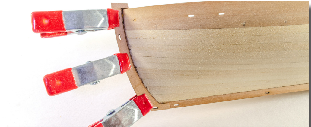
81. Glue both parts #49 to the prow, as shown, one on each side. Make sure the locating peg holes are aligned.
