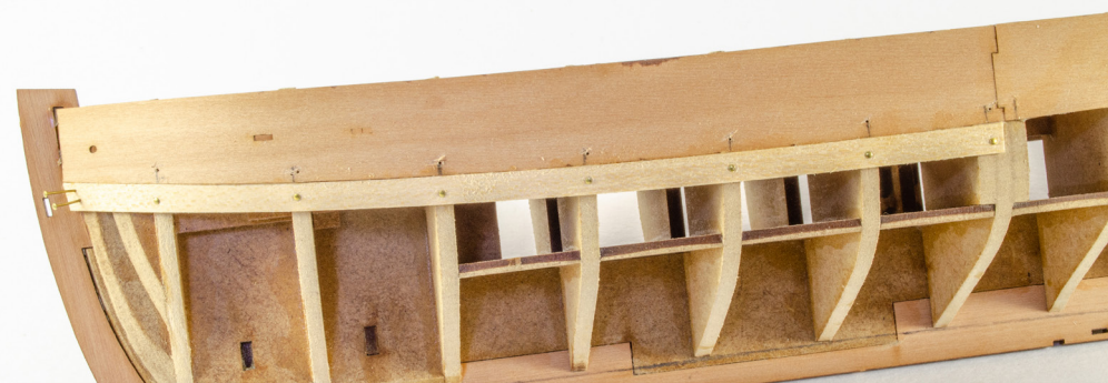
67. It's now time to start adding the first layer of lime planks. Take of the wider and thicker lime planks and glue it immediately underneath the bulwarks. This does not need to be tapered. You can also install the plank in halves if you wish, as we have done here for you. Remember to pin the planks and also glue them to each other along their length.
