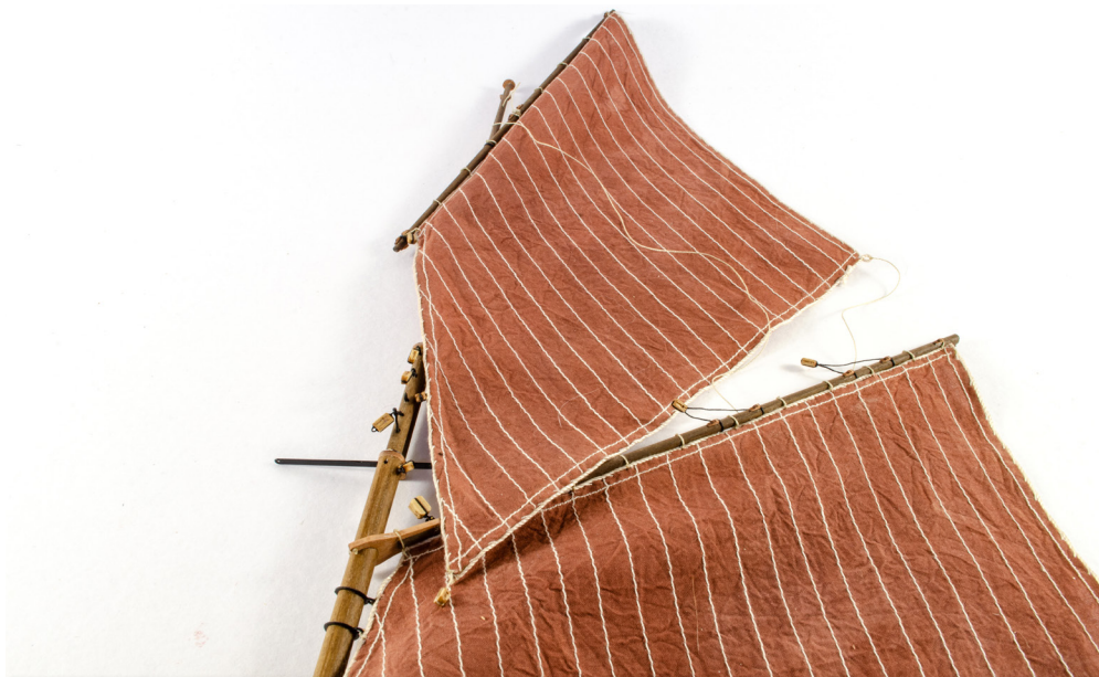
217. The main topsail yard can now be lashed to the top of the mast as shown here and on plans.
