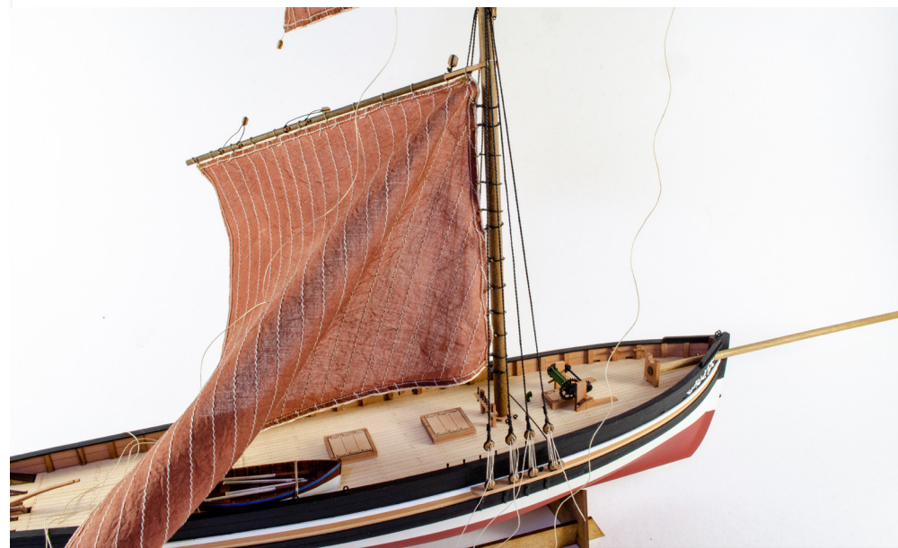
220. 3mm deadeyes are now added to the shroud lines and then 0.1mm natural thread is used to rig the lanyards.
