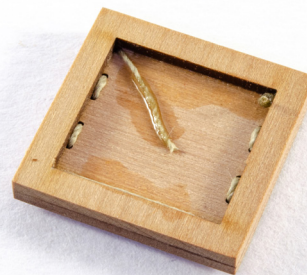
158. Cut short the thread here and use CA to glue it to the underside of the hatch.
